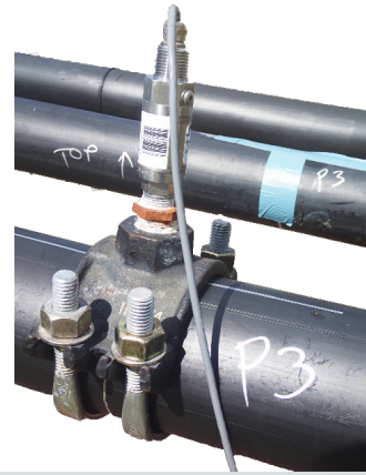
Figure A7. Typical pressure transducer and pipe saddle on tendon.
