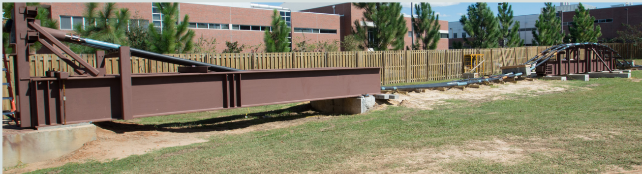
Figure A1. Tendon profile for the mock-up testing on unbonded tendons.
