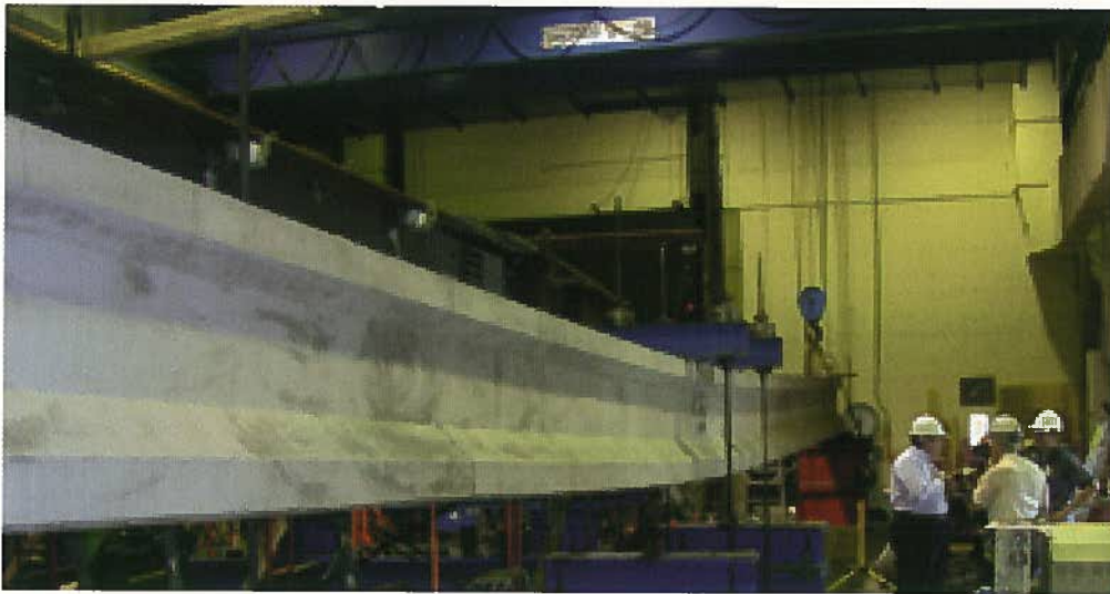
In the laboratory, the UHPC girder deflected approximately 12 in. (305 mm) without showing any visible cracks.
