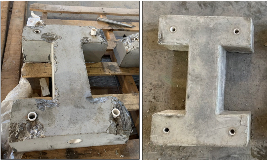
Figure 9: I-shaped tile before greasing forms and caulking joints (left); I-shaped tile after greasing forms and caulking joints (right).
