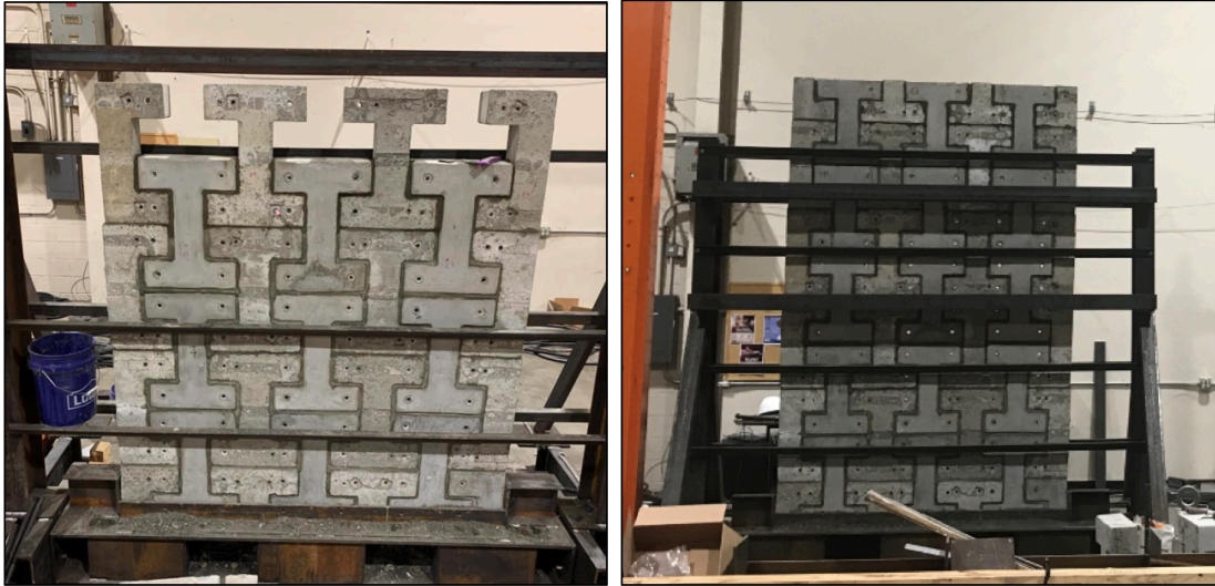
Figure 12: Each successive row could be slid into place by adding and removing angles during construction process (left); Fully stacked wall (right).
