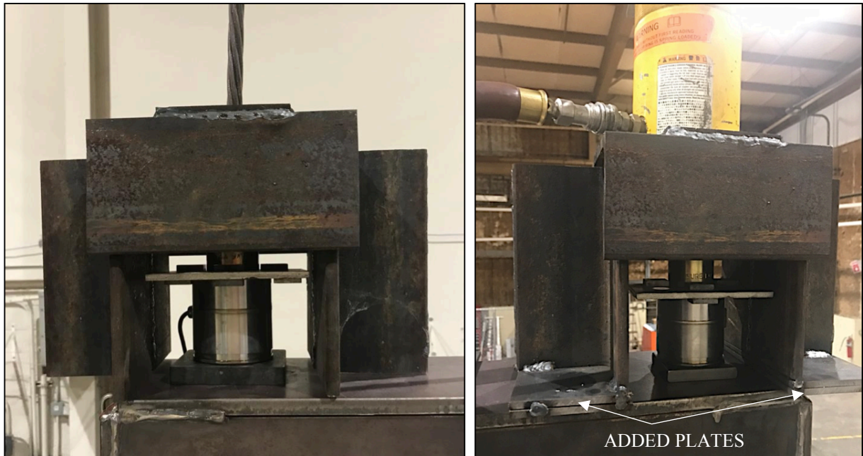
Figure 14: Steel saddle at edge before adding supporting plates to bottom (left); strand jacking setup with supporting plates added to saddle (right).
