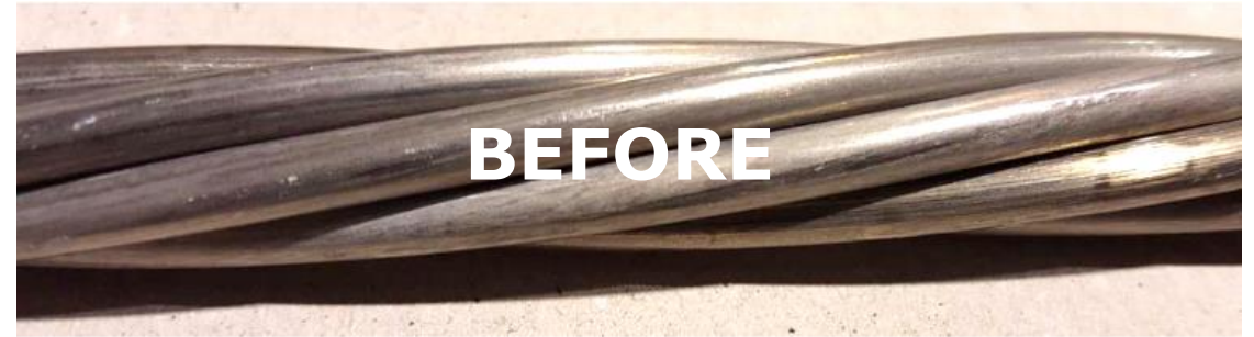
Figure 1 Specimen Surface Conditions prior to the Salt Fog Test
