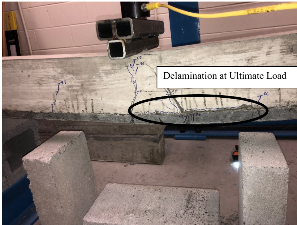
Fig 10 Laminate2 beam cracking pattern at ultimate load with delamination.
