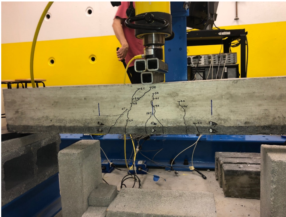
Fig. 9 Laminated beam cracking pattern at ultimate load without any delamination.
