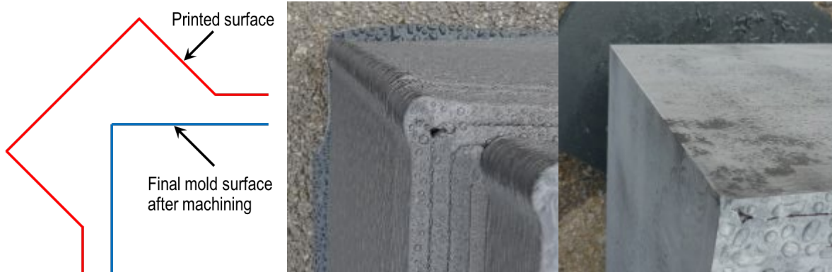
Figure 22. Overrun or extra material printed at corners (left image) so that the “corduroy” finish (middle image) can be machined to generate the desired corner shape (right image).
