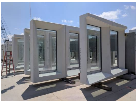
Figure 35. Pre-glazed panel at production yard ready for shipment
