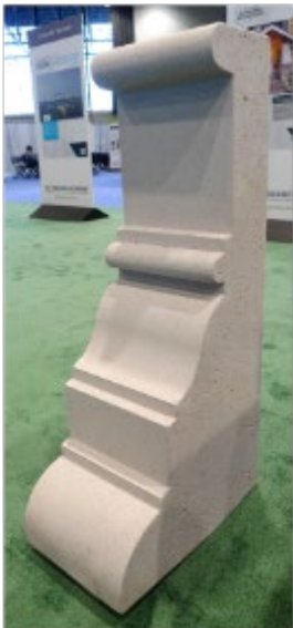
Figure 8. Precast cornice cast by Gate Precast using the prototype 12-inch deep cornice mold.
