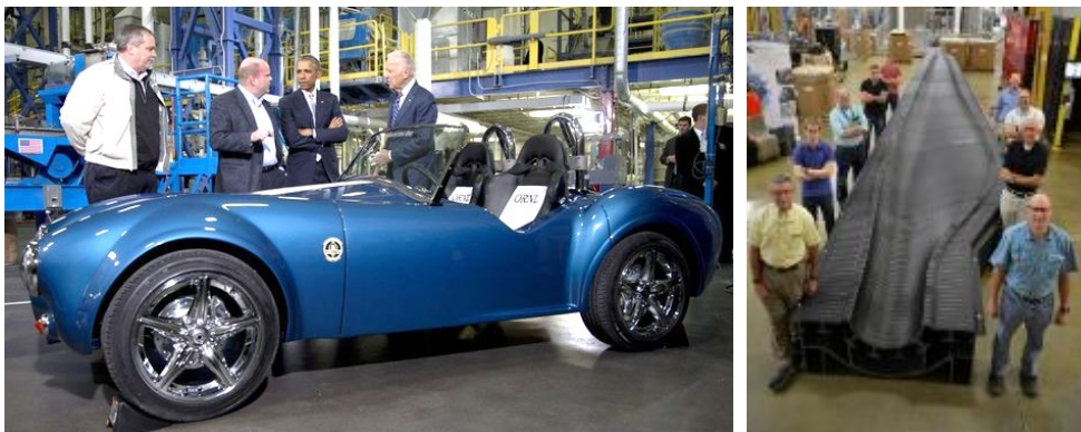
Figure 3. 3D printed Shelby Cobra (right) and mold for wind turbine (left).
