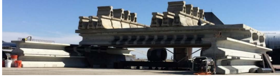
(b) test bridge loaded with the simulated AASHTO design truck load
