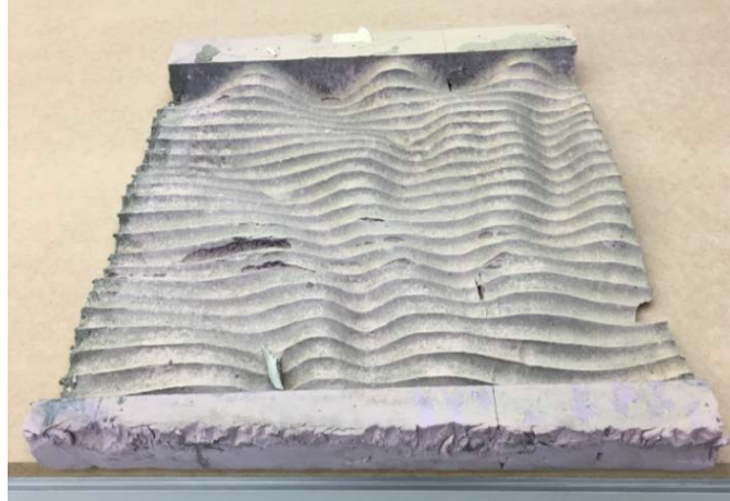
Fig. 2- A sample of printed formwork to make an aesthetic concrete surface
