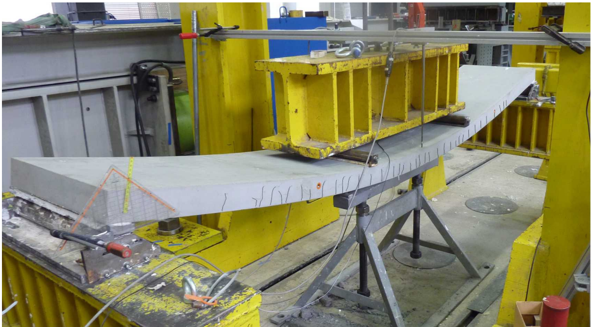
Fig. 10: Carrying out the experiment of the four-point bending test and crack image just before the break
