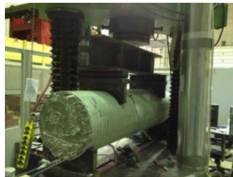
(a) 203.2 mm diameter specimen during test (b) 304.8 mm diameter specimen before test Fig. 2: Instrumentation of concrete column specimens under axial compression
