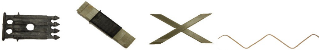
Figure 2 – Shear Connectors Tested, Left to Right: THiN Wall NU-Tie, HK Composite Tie, Thermomass CC and Thermomass X
