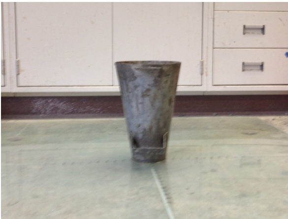
Figure 1. Slump flow test setup using Procedure B of ASTM C1611 9 .
