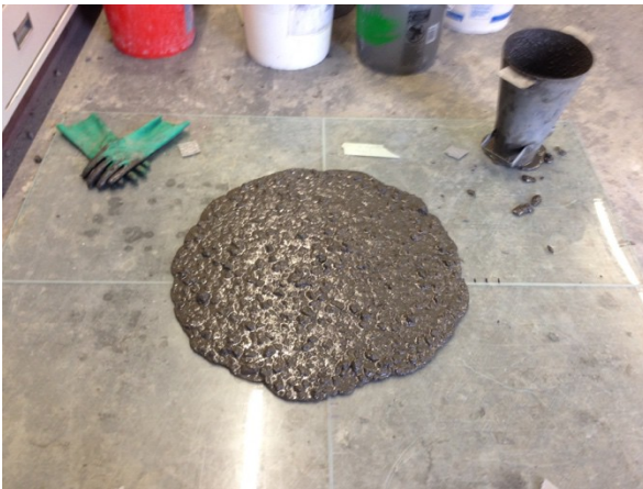
Figure 2. Slump flow test sample once allowed to flow completely per ASTM C1611 9 .
