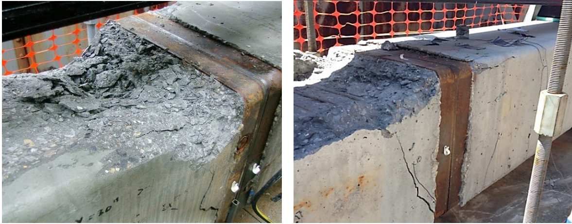
Fig. 10 – Failure of compression zone of Test 1 (left) and Test 2 (right)
