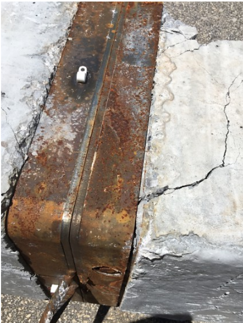
Fig. 11- Gap between splice assembly and the concrete in Test 2
