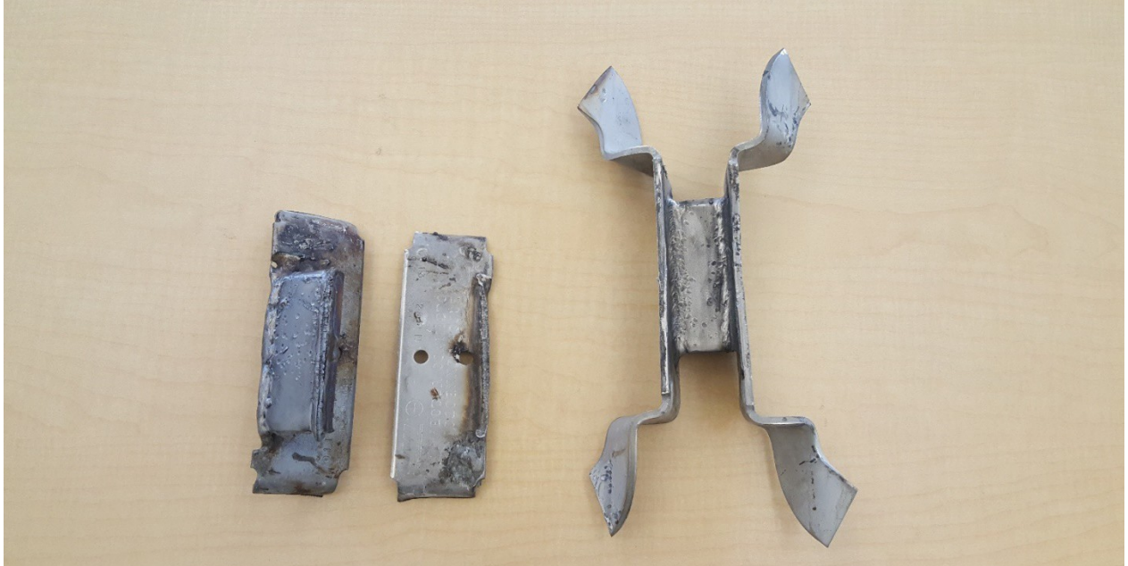
Figure 10: Flange connection hardware extracted from parking garage
