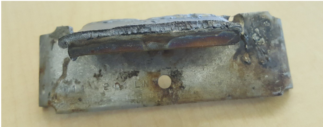
Figure 11: Inadequate weld to base metal penetration observed at failed weld location
