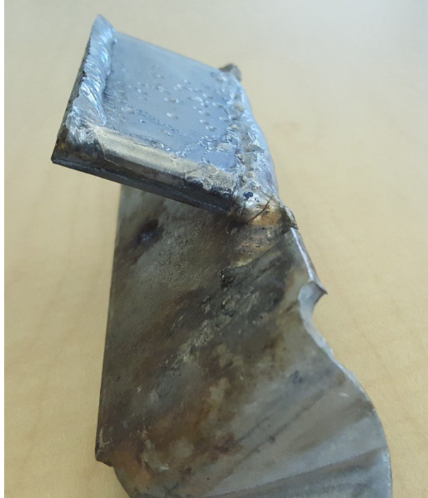
Figure 12: Crack at end of intact weld
