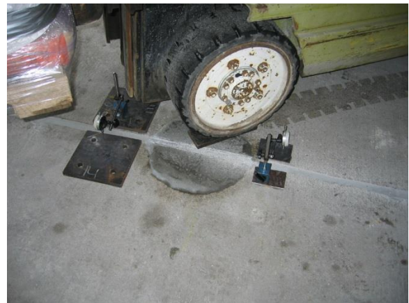
Figure 19. Close-up view of load test on core-hole repair
