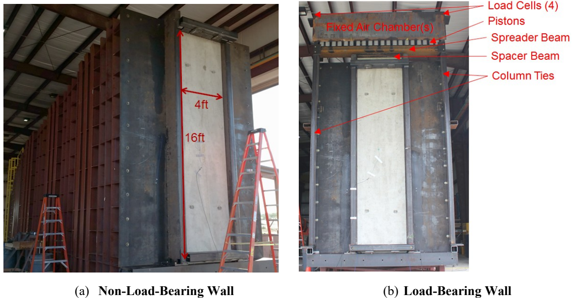
Figure 2. Wall Specimens Mounted in Shock Tube
