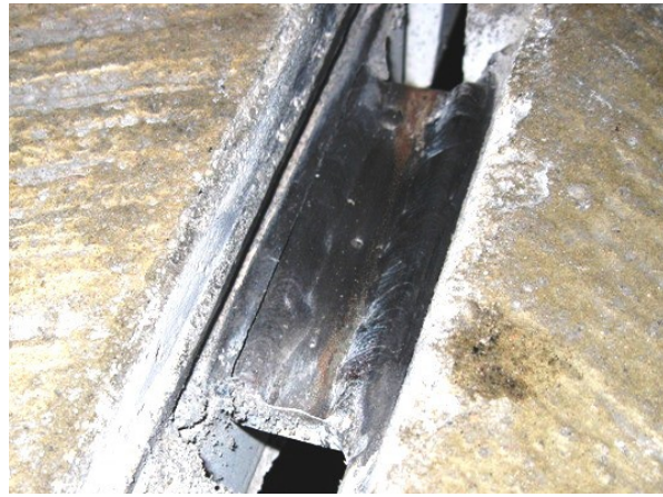
Figure 4 Fatigue failure of flat bar-type connection.
