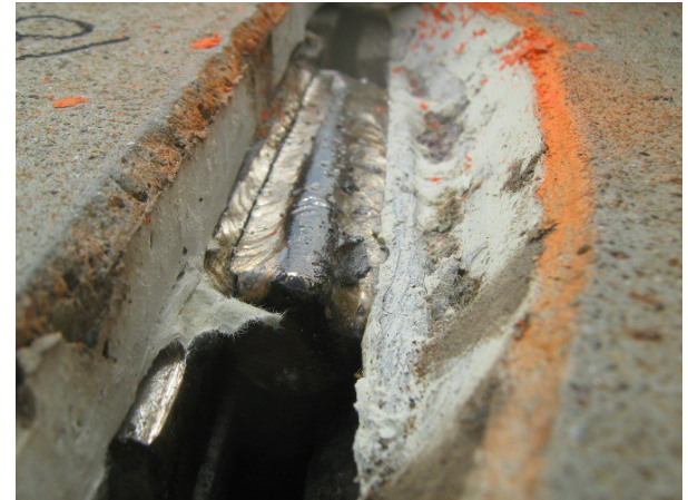
Figure 5 Fatigue failure of flat bar-type connection.
