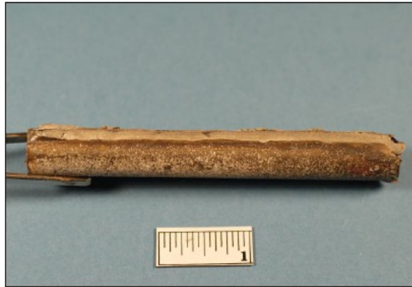
Figure 10A Fatigue failure of a dowel-type connection.
