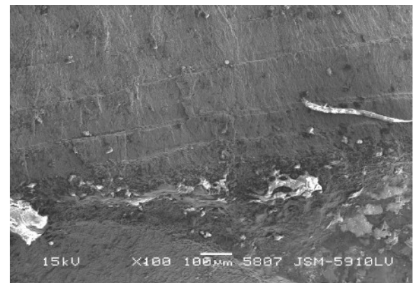
Figure 11B Fatigue failure of a flat bar-type connection; scanning electron micrograph.
