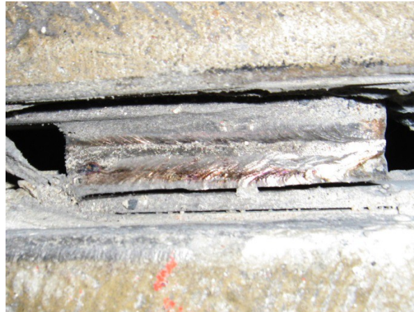
Figure 4 Fatigue failure of flat bar-type connection.
