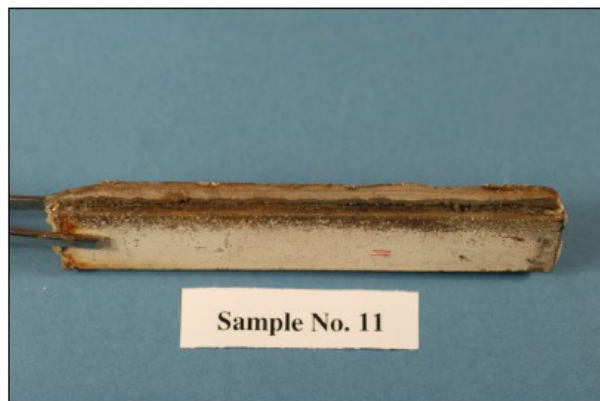
Figure 11A Fatigue failure of a flat bar-type connection.
