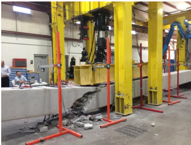
Fig. 20. Failure under one of the load points
