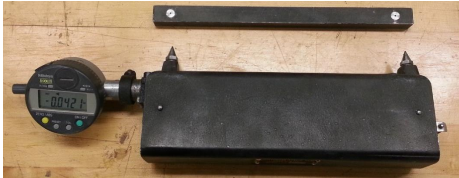
Figure 7: Whittemore gage with 8-inch gage length was used to obtain surface displacements
