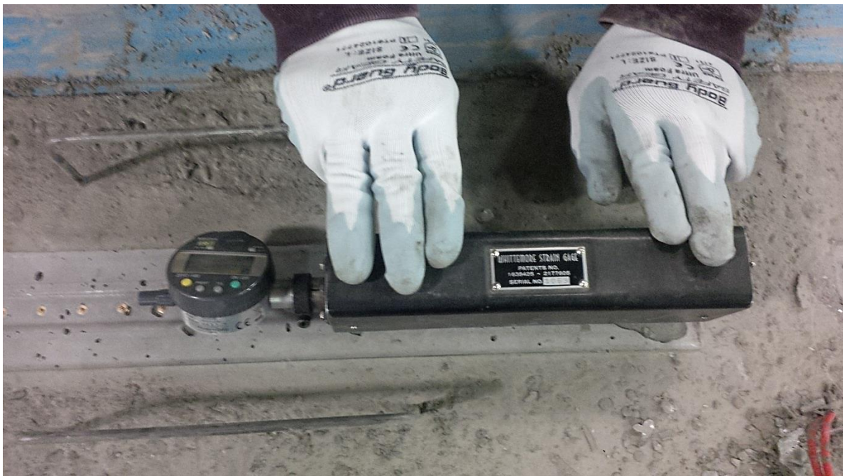
Figure 8: Distance measurement between brass inserts using Whittemore gauge
