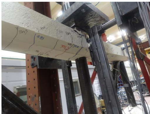
(a) Crushing of Top Chord
