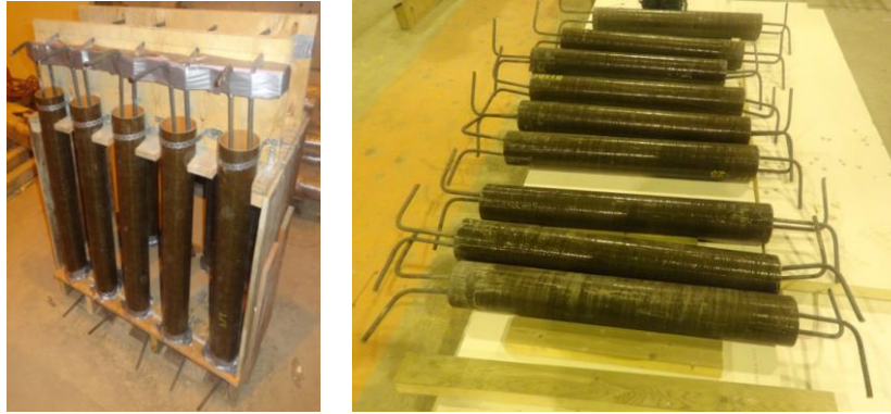
Fig. 5 The vertical truss elements before and after casting
