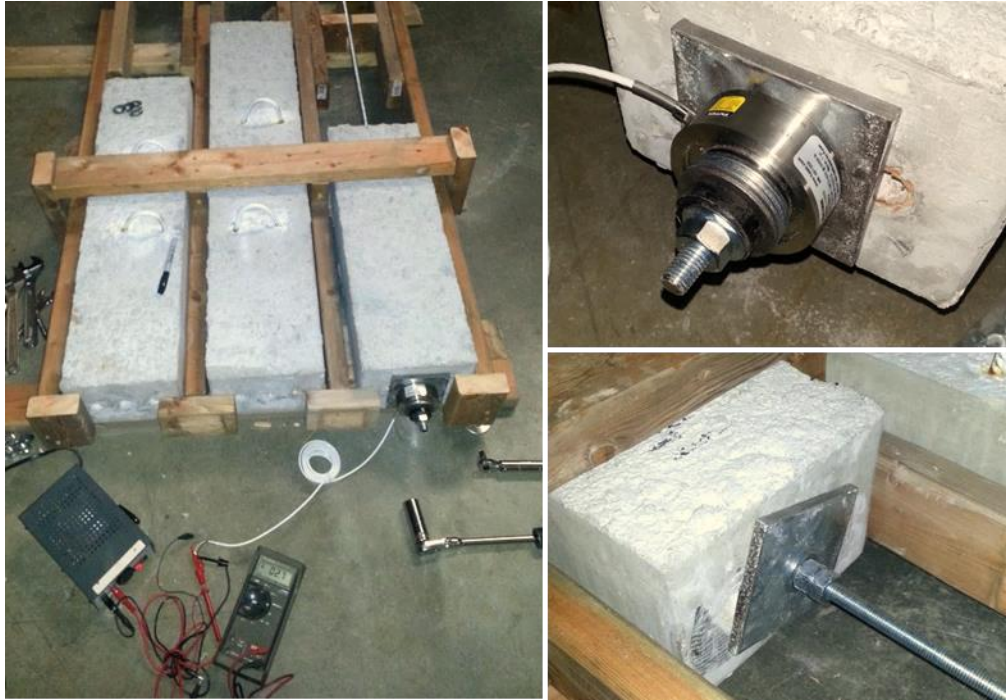
Figure 3. Test frame and data acquisition (left) and bearing details for the live end (top right) and anchor end (bottom right)
