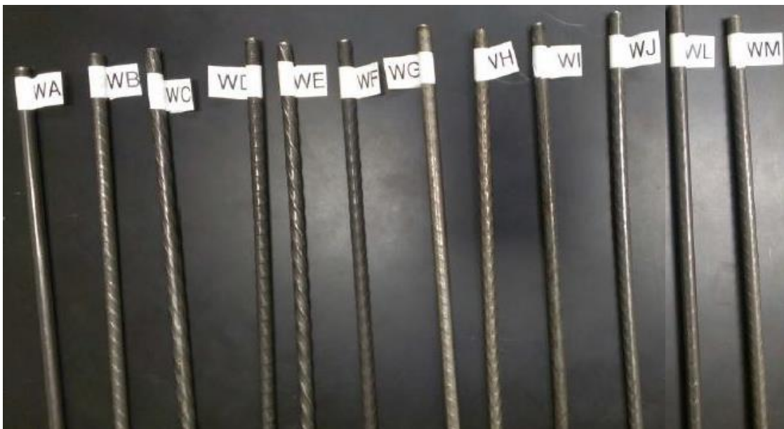
Figure 1 : Twelve different 5.32-mm diameter prestressing wires
