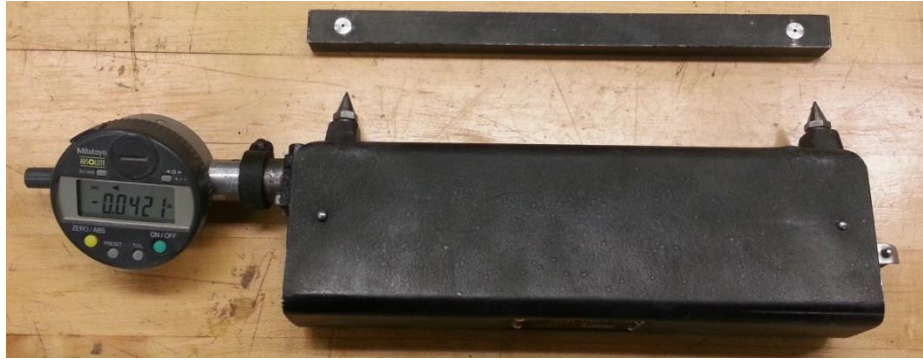
(a) 8-inch gage whittemore gage used for strain measurements
