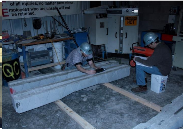
(c) Distance measurement through whittemore gage after detensioning
