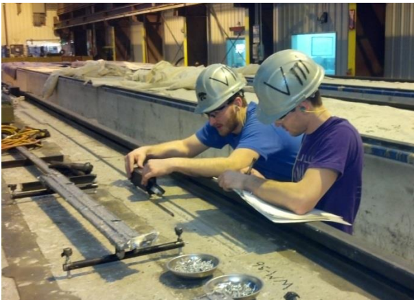
(b) Distance measurement through whittemore gage prior to detensioning
