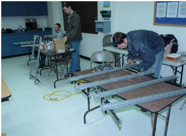
(a) Brass inserts mounted on steel bar at one inch spacing
