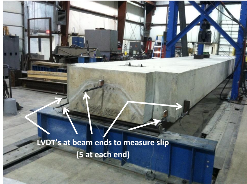
Figure 7. Location of LVDT's at the ends of the composite beam to measure slip.
