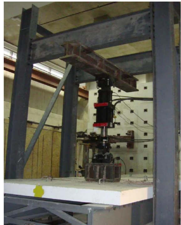
d) Test setup for fatigue testing
