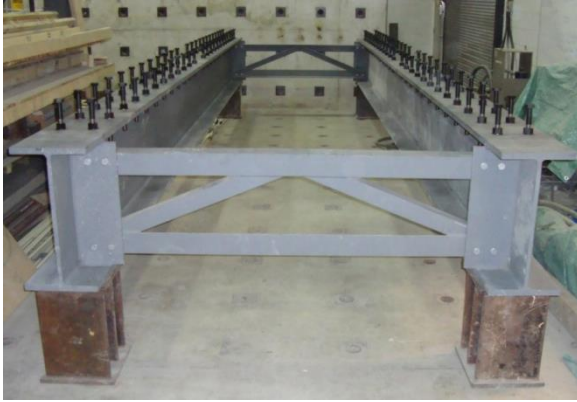
a) Twin-girder assembly and shear connectors
