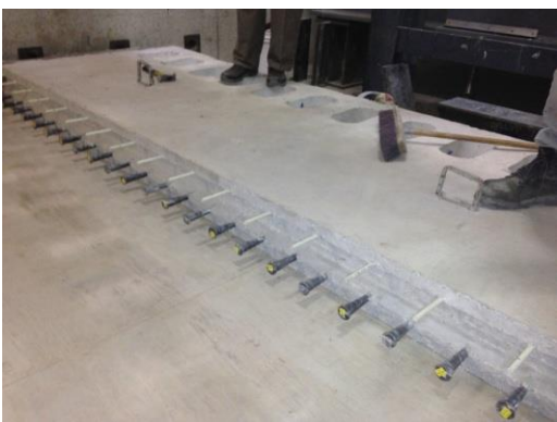
b) GFRP bars and styrofoam forming the joint
