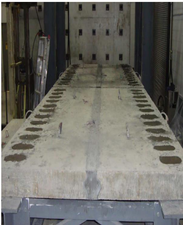
c) Precast jointed-slab before loading
