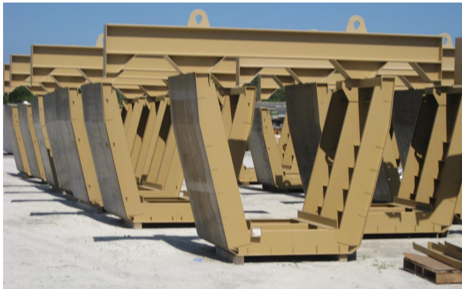
Figure 12: U-Girder Interior Form Sections
