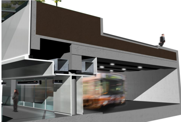
Figure 7: Partial Section of the Underground Bus Terminal.
