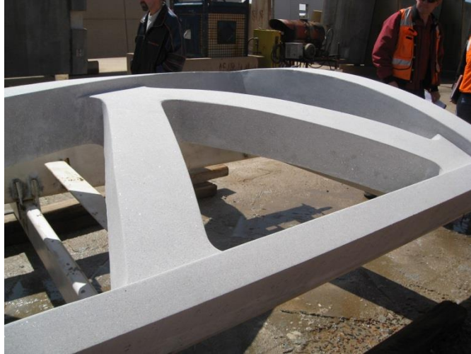
Figure 31: Precast vent towers at the precast plant after casting.
