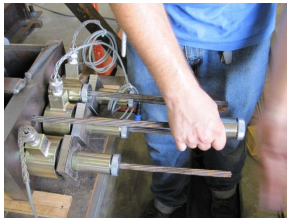
Figure 11 – Chucks and load cells at unbonded segment end
