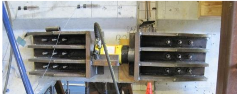
Figure 10 – Extend plunger of hydraulic jack
