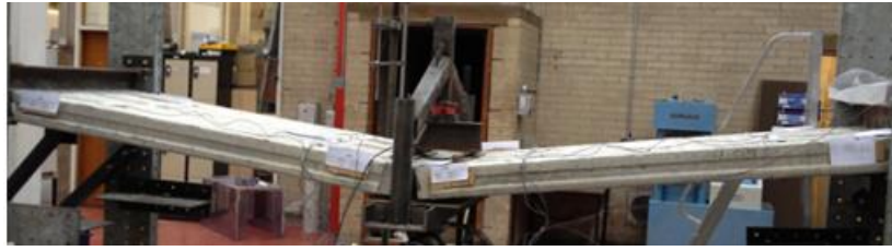
Fig. 8 Failure pattern of test assemblies
