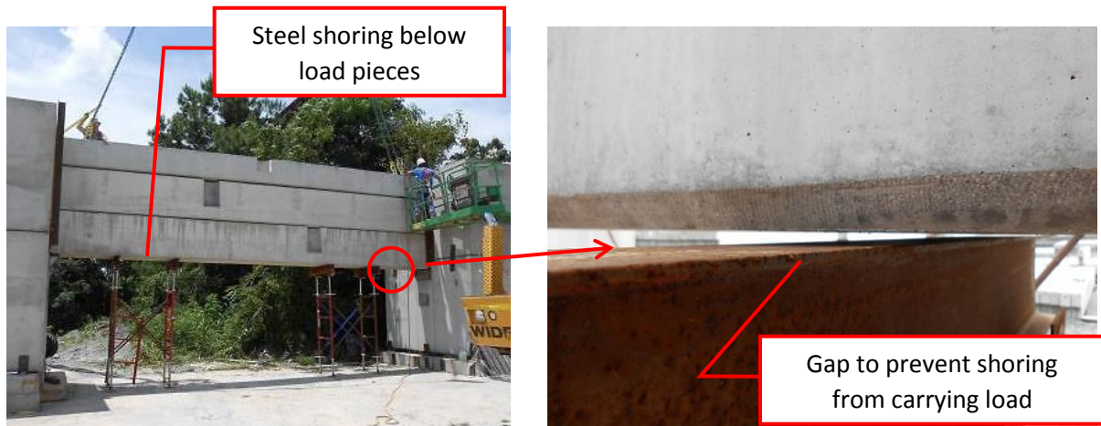
Figure 4 - Shoring below precast member during testing
