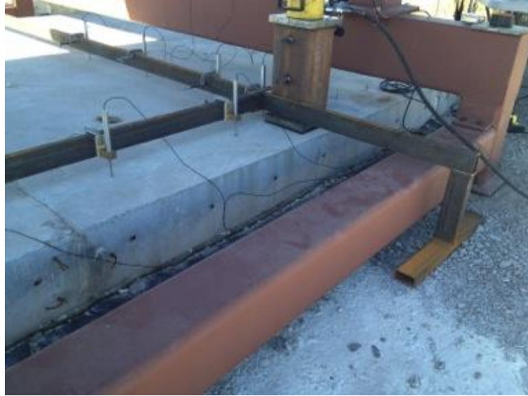
Figure 14 Instruments and loading at the 10 in. pavement at location 3.
