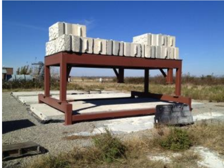
Figure 13 Steel frame assembled and ready for testing
