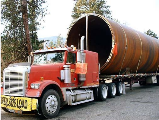
Figure 5 Over-height load that damaged the Easton Road Bridge
