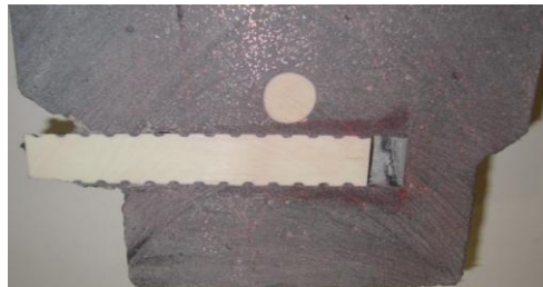
(e) Bar slippage from the head in slab S6
