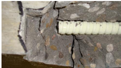
(a) Bar debonding in slab S3
