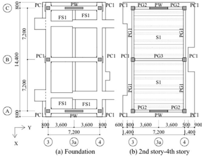
Fig. 2 Plan View of the Specimen (Unit: mm)
