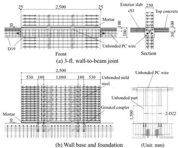
Fig. 4 Reinforcement Details of Walls (Unit: mm)
