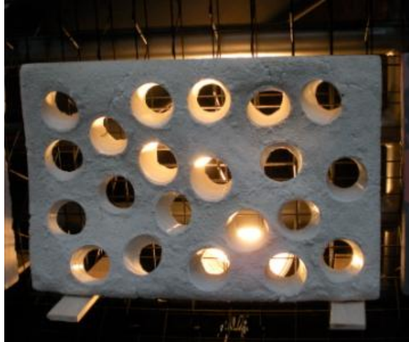
Fig. 16 Panel was contour formed in a sand bed with embedded plastic cups, which can be popped out and reused.
