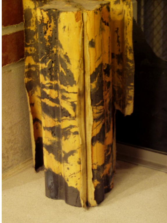
Fig.10 The dye pattern was absorbed into the paper formwork which created a negative image of the pattern.
