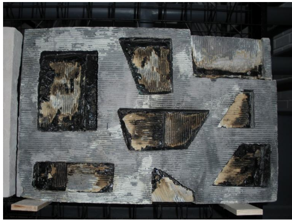
Fig. 23+24 This student learned that corrugated cardboard is inexpensive as a form liner, but quite labor intensive to strip the form.
