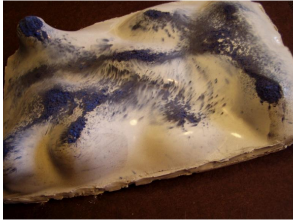
Fig. 13 Color dye that is not fully mixed gives an interesting texture on this slick formed panel.
