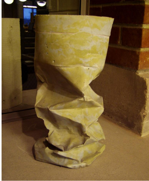
Fig. 22 The creases at the bottom of this crushed cylinder form are paper-thin.
