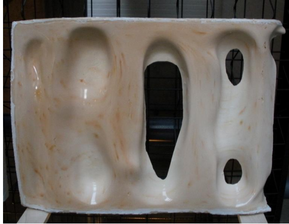
Fig.14 A slick finish pastel panel illustrating a variable thickness from 2" to 0" The edges around the holes are paper-thin.
