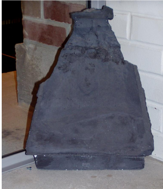
Fig.25 Two sides of a plywood box were filled with a block of ice of variable thickness. Due to the heat of hydration, the form was self-stripping.
