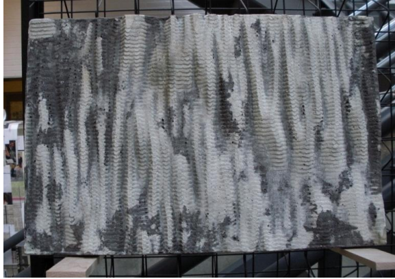
Fig.11 This simple white/charcoal color mix that was cast on a piece of rigid insulation board that had been distressed with a dinner fork prior to casting.
