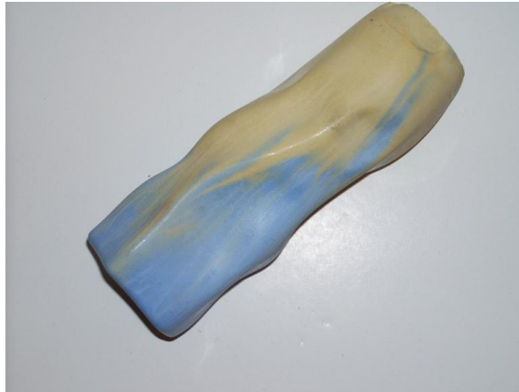
Fig. 8 A bi-color mix poured in a cylinder started out as a pastel blue, was rodded and a tan pastel mix added on top to complete this pour.
