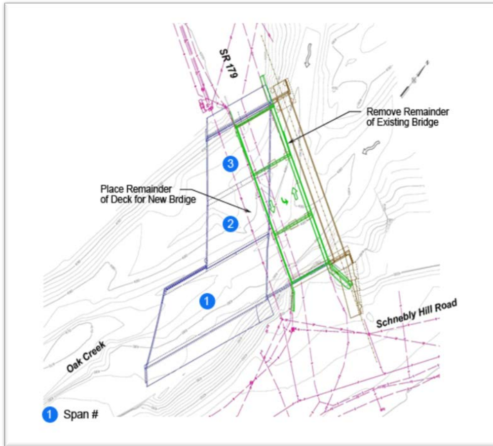
Fig. 9: Phased Bridge Construction (Phase 2)
