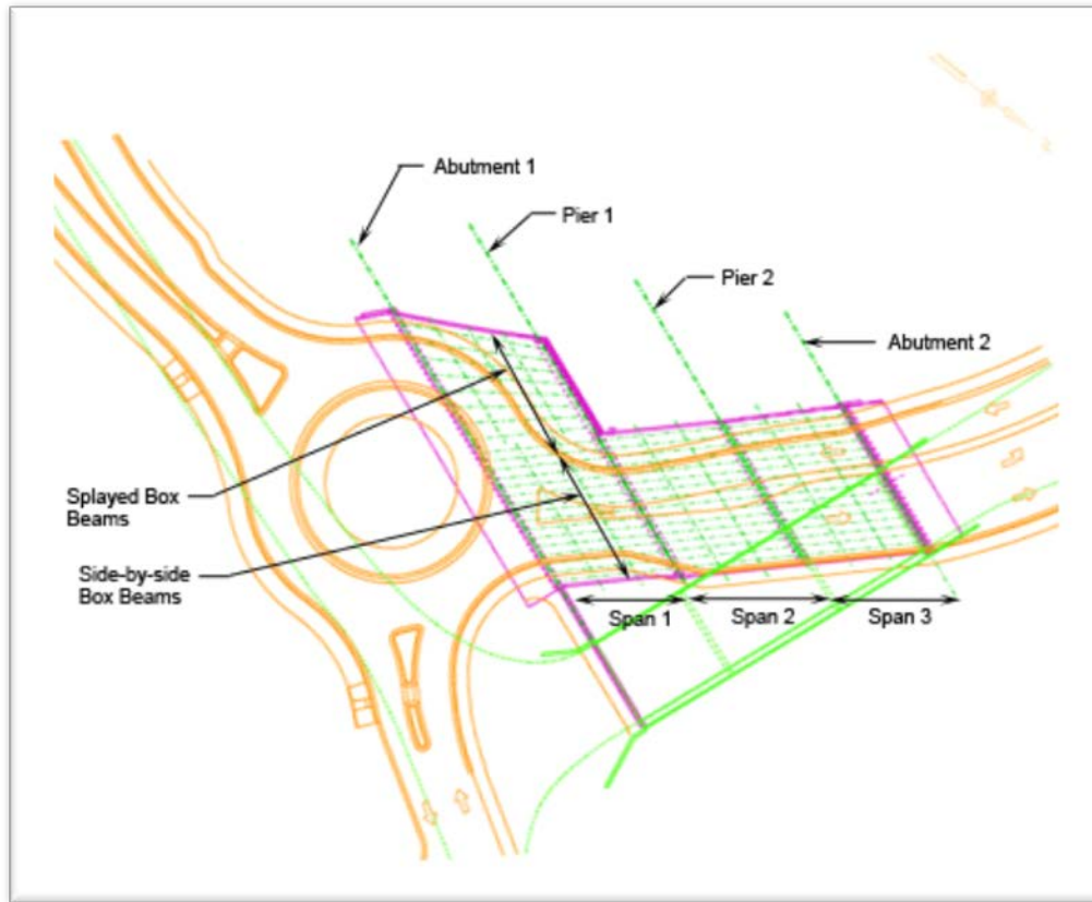
Fig. 5: Superstructure and Substructure Configuration
