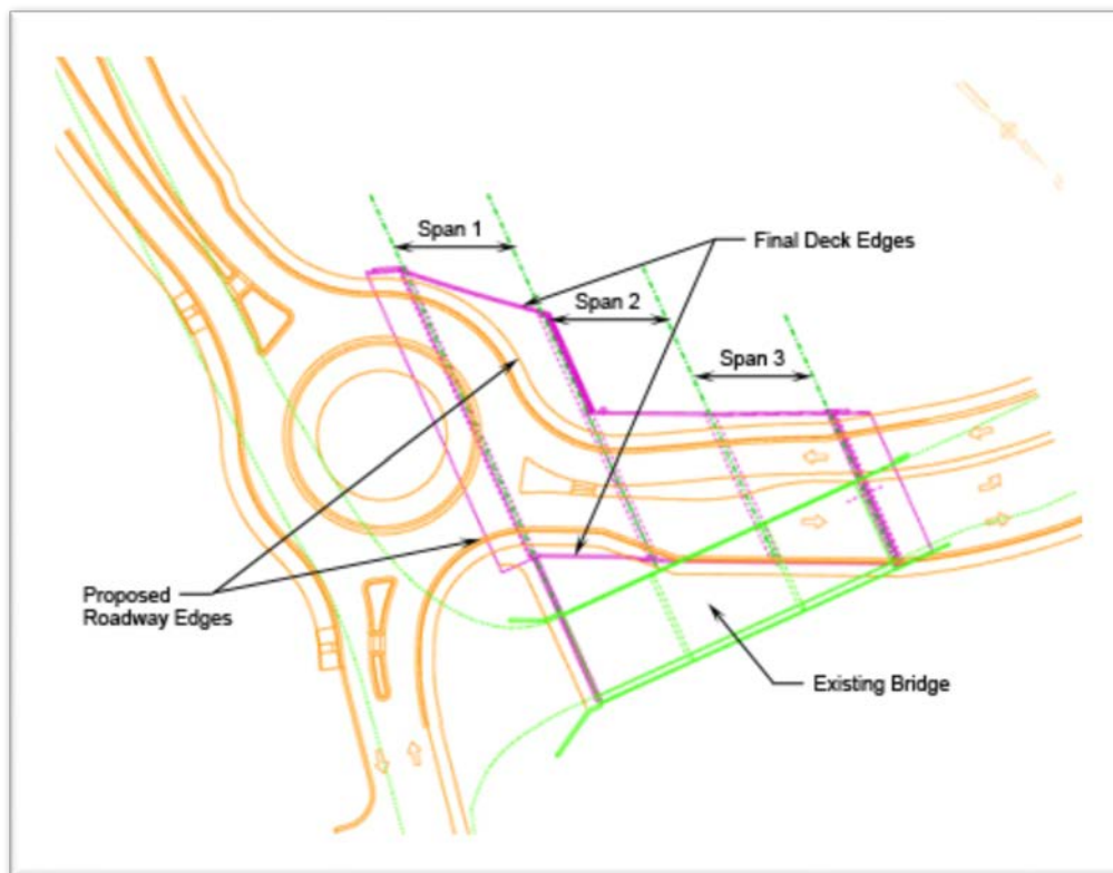
Fig. 4: Proposed Roadway Configuration at Existing Bridge
