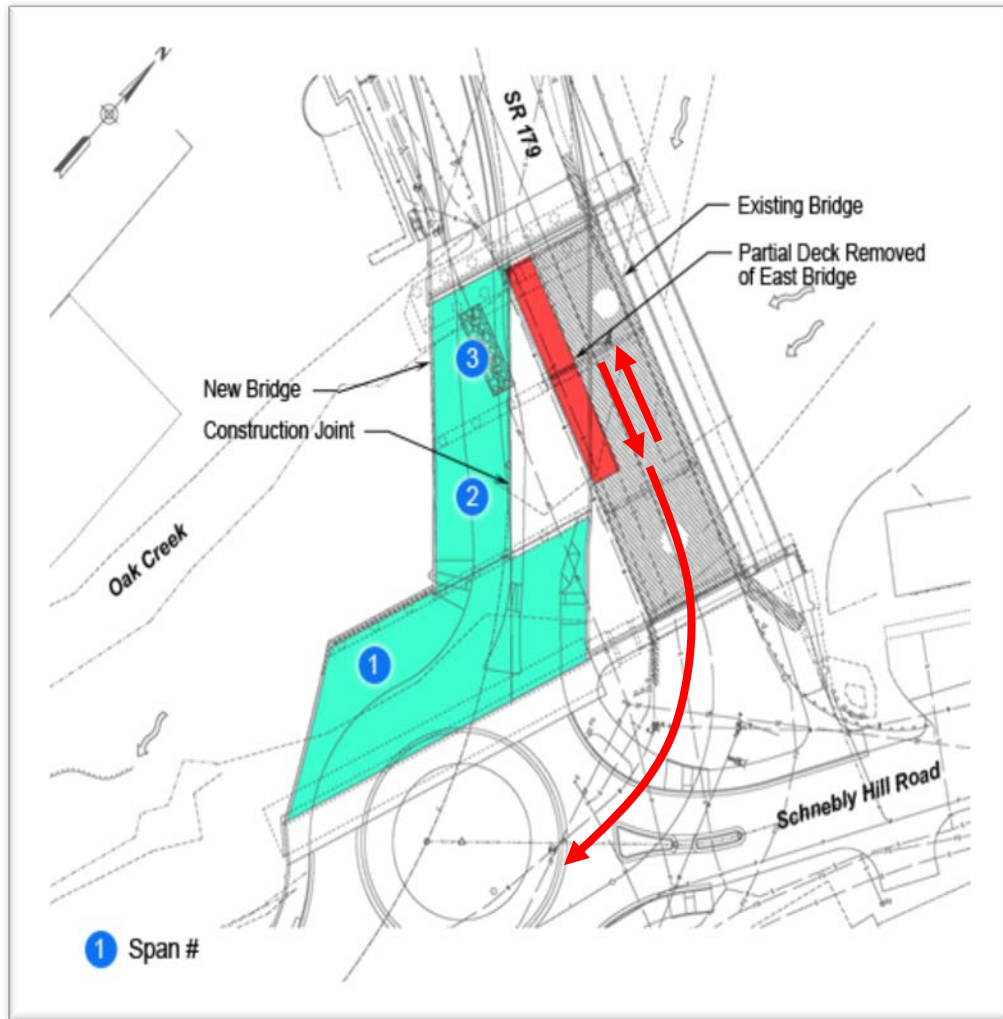
Fig. 8: Phased Bridge Construction – Phase 1
