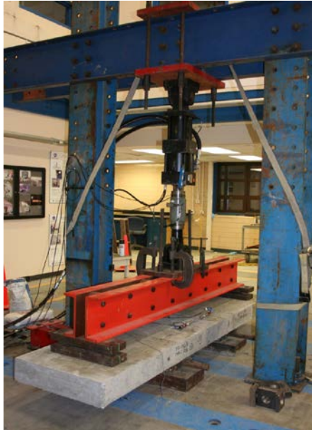
Fig. 3 Deck-level connection specimen test setup.
