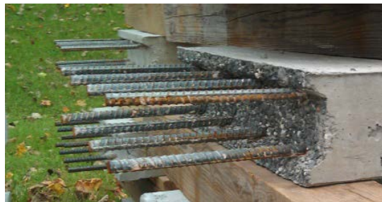
Fig. 2 Trapezoidal shear key with exposed aggregate surface.
