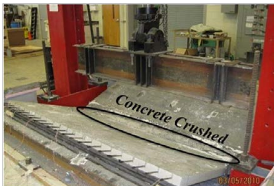
Figure 2 Typical Flexural Failure at Midspan by Concrete Crushing of Simply Supported Panels (Panel ST-NC-SL shown)
