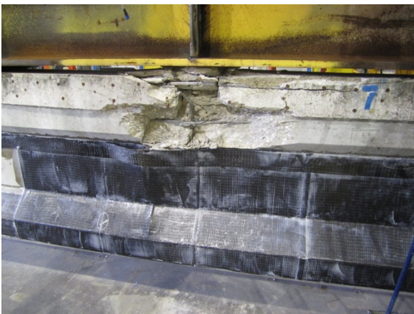
Fig. 27-b: failure shape mode of full scale PSC beam by static testing
