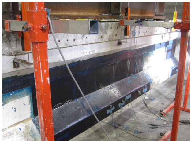
Fig. 27-b: failure shape mode of full scale PSC beam by static testing
