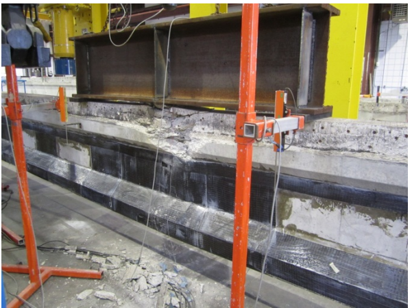
Fig. 27-a: failure shape mode of full scale PSC beam by static testing
