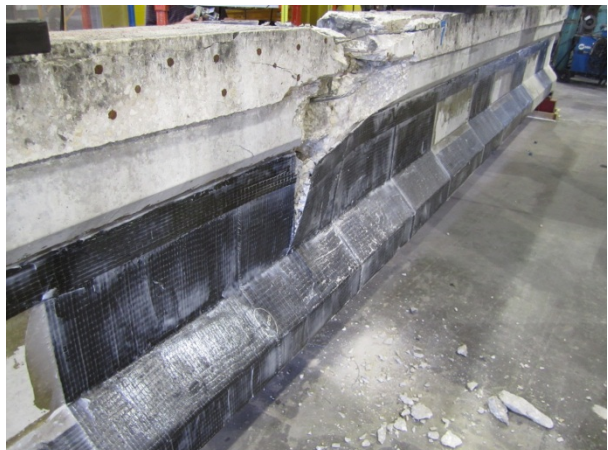
Fig. 27-a: failure shape mode of full scale PSC beam by static testing
