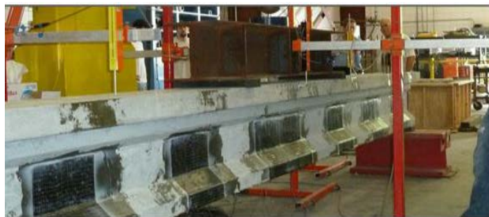
Fig. 5: Half Scale girder test setup during testing
