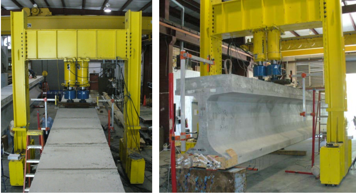
Fig. 4 Test Specimen in Load Frame
