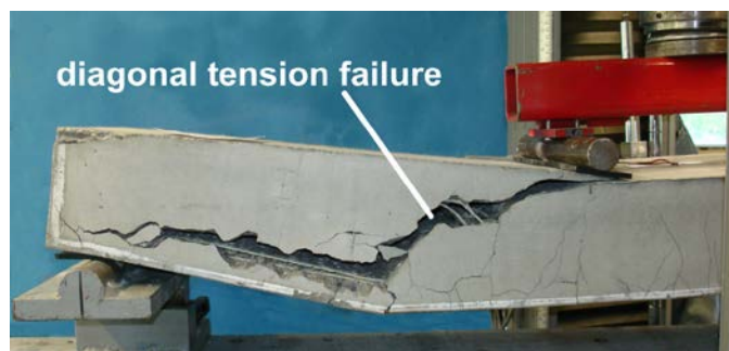
Fig. 9 Failure mode of the slab-test
