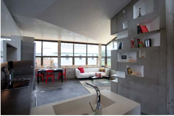
Figure 27: Interior view looking south of the completed eNJoy! House in West Potomac Park, Washington, DC, September 2011. The interior utilized a dark-tinted precast floor panel, naturally finished wall panels, and a roof painted with gloss white epoxy.
