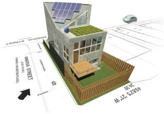
Figure 4: Preliminary rendering of PREttyFAB showing the photovoltaic array and green roof at the rear of the house – within the 30-foot rear yard setback.
