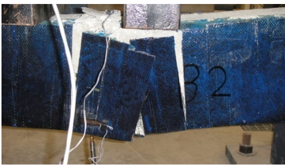
(c) CFRP debonding B2 set #2
