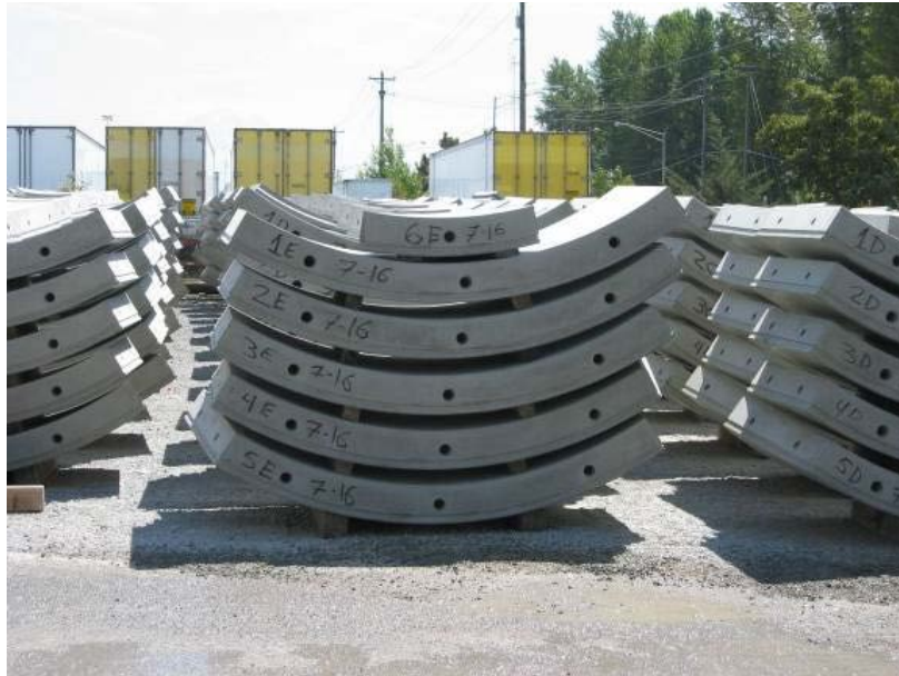
Figure 4: Concrete precast ring panels 9 .
