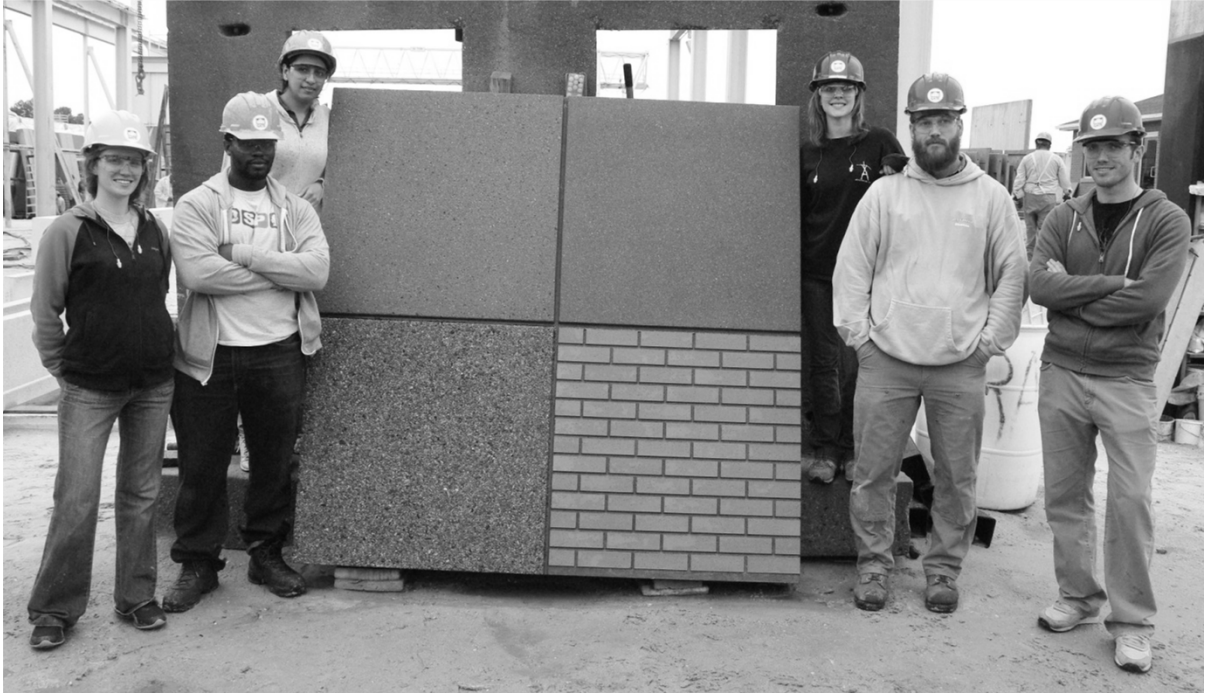
Fig. 3 Student team with the architectural precast concrete sample panel they fabricated.
