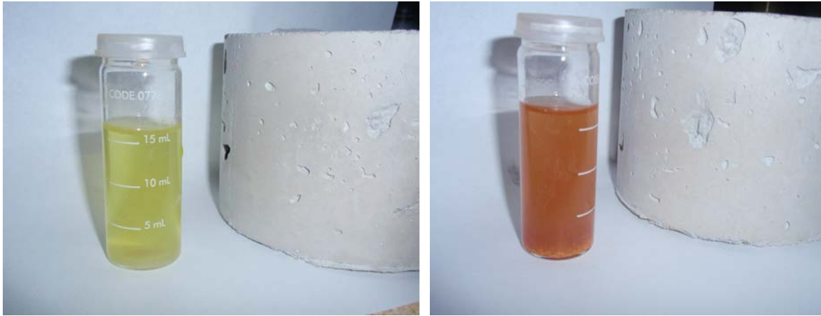
FIG. 11 w/ Potassium Chromate (Light Yellow) FIG. 12 end-point color (Orange Brown)
