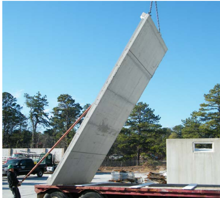
Figure 7: Handling the 20 ft long test specimen
