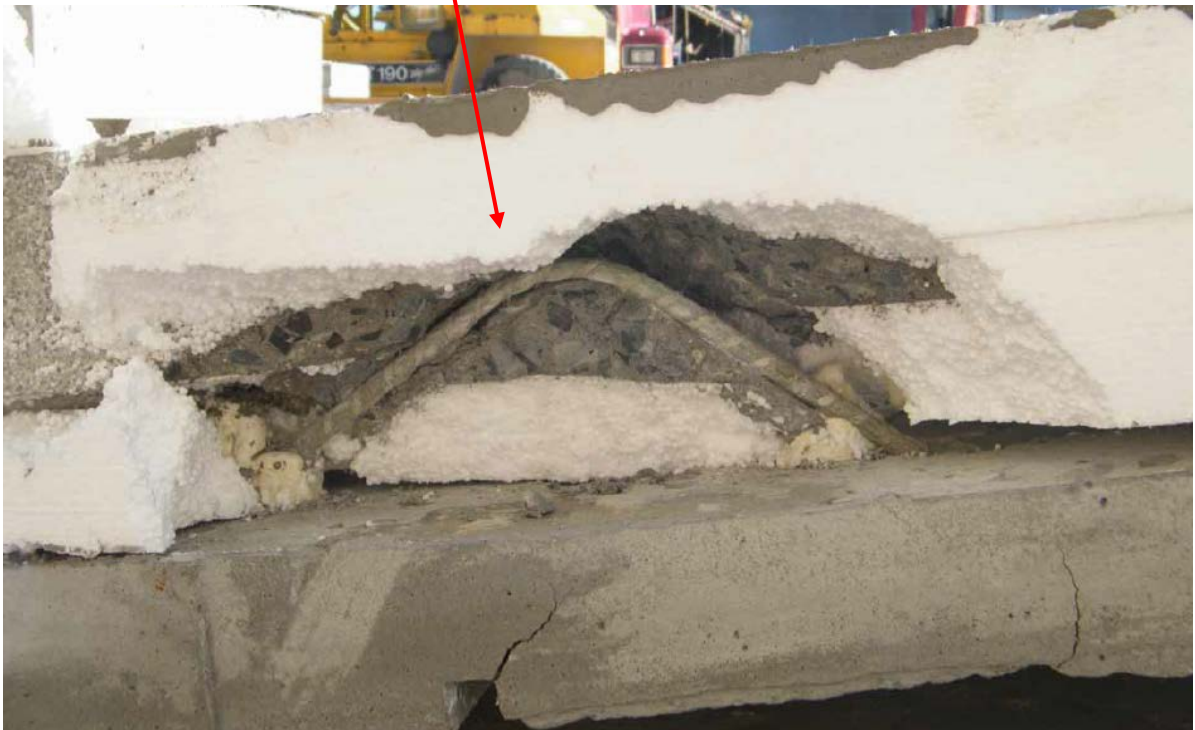
Figure 12: Horizontal shear failure of the 16 ft long panel due to the pullout of GFRP ties
