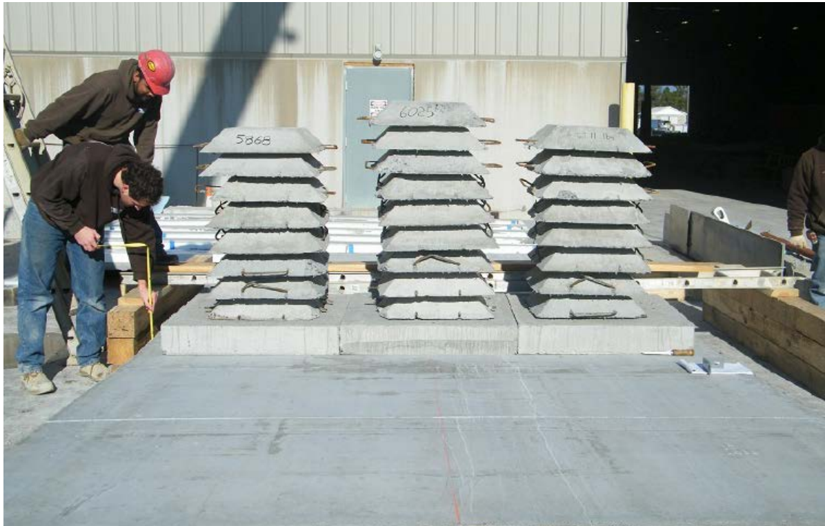
Figure 9: Loading the 20 ft long specimen on the flat side
