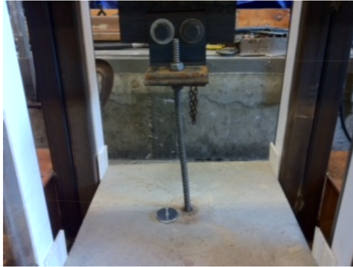
Figure 5. Component Testing of Flexing Coil Rod Connections
