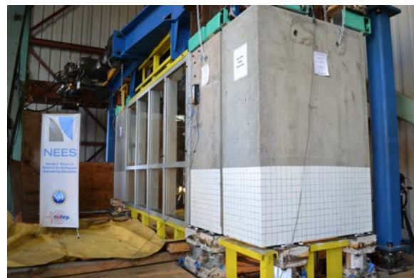
Figure 2. Exterior Face of Precast Concrete Cladding Panels before Experimental Testing
