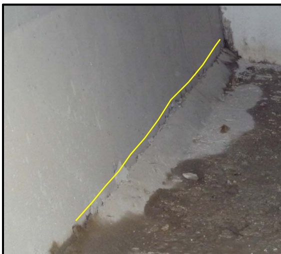
Figure 6: Horizontal cracking visible at the bottom flange-to-web interface on the inside of test specimen B2N.
