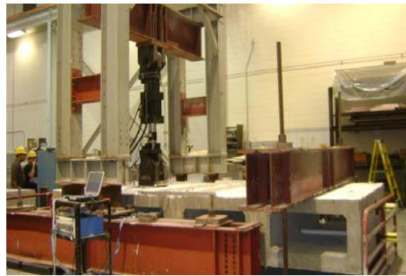
Fig. 13 Actuator at Exterior Joint for Top Tension Setup
