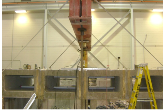
Fig. 15 Actuator at Interior Joint for Ultimate Capacity Setup
