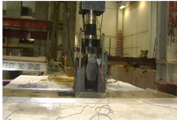
Fig. 14 Actuator at Interior Joint for Bottom Tension Setup
